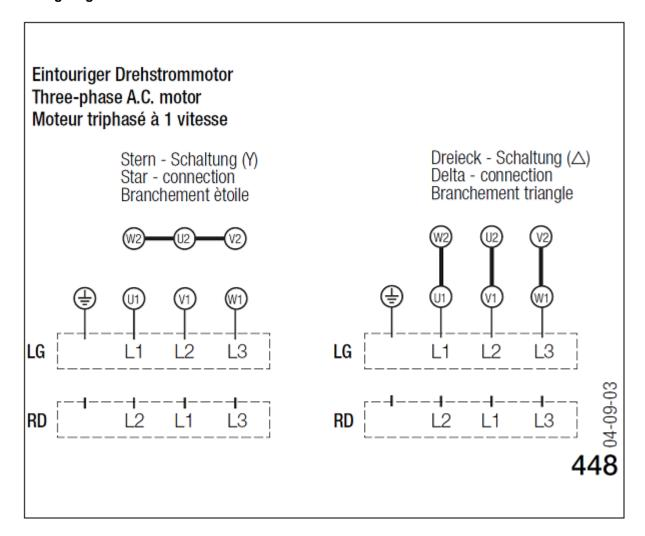
Wiring diagram for connection to: mains - motor Rotation: RD
